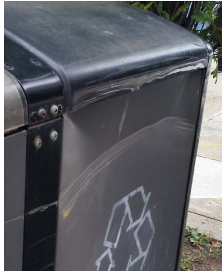
7 th & Arch NW, Cracked Solar Bubble and missing screws and rear panel damaged, September 20, 2016
