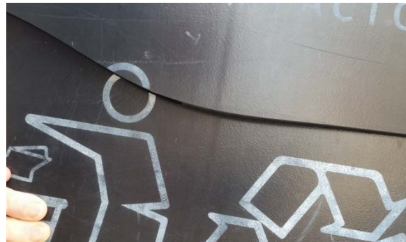
Additional cracks in Solar Bubble and on side of container. 7 th & Arch, August 8, 2016
