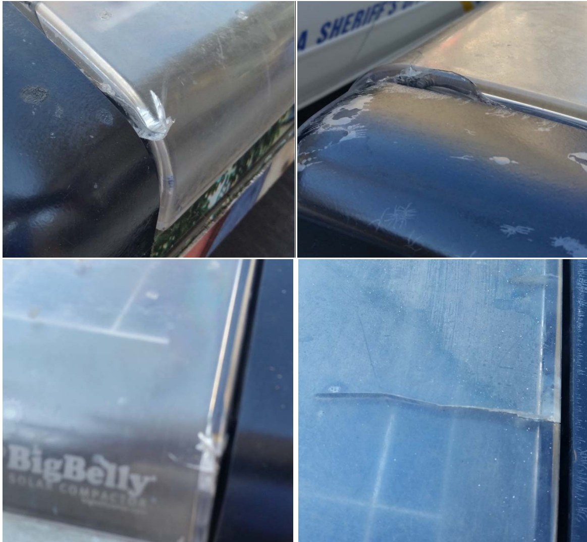
Solar Bubble cracked in four places, Broad & Arch, August 5, 2016
