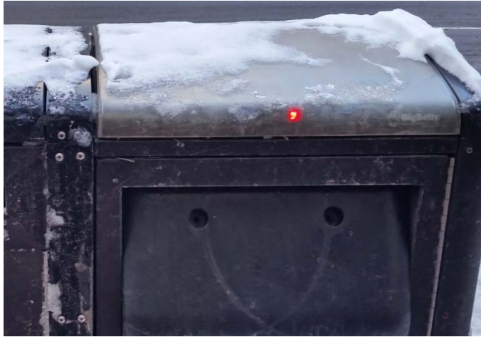
Handle missing, unit not functioning, Juniper & Market March 16, 2017. Handle still missing as of June 7, 2017.
