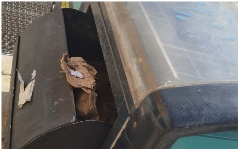
Many units had cracked solar bubbles and rusted rivets, as noted here at Broad & Callowhill on July 14, 2016
