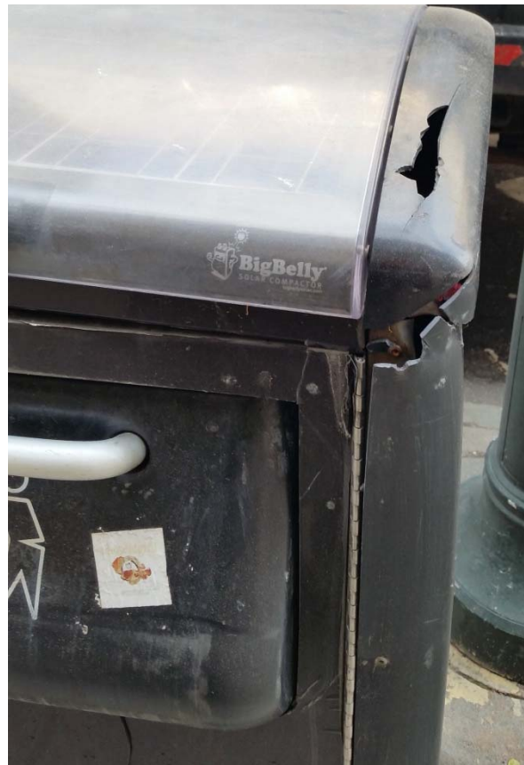
Severe damage, door not properly aligned, 12 th & Chestnut, February 15, 2017
