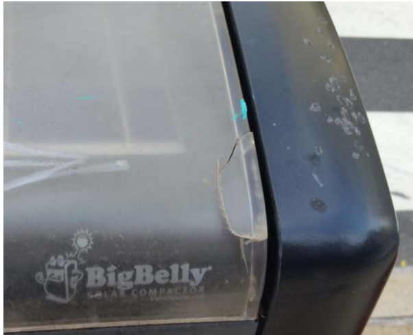
Additional cracks in Solar Bubble and on side of container. 7 th & Arch, August 8, 2016
